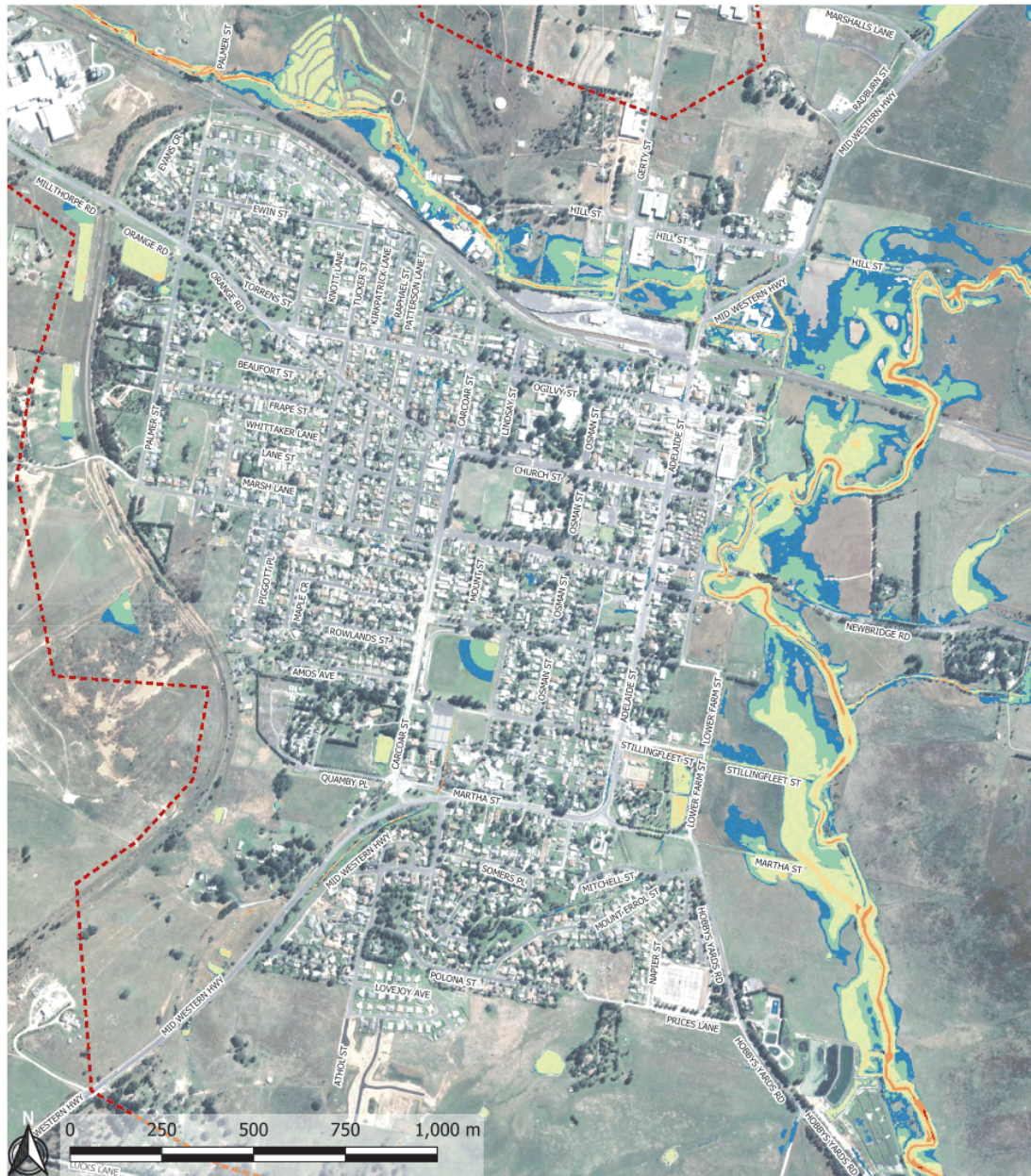
Map 07: Proposed With Basins Flood Hazard 20% AEP Event (ARR 2019)
