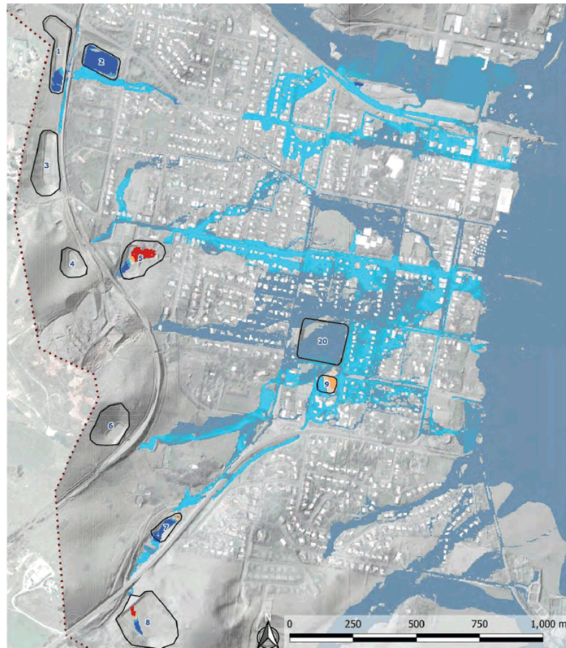
Figure C100-2: Flood Level Difference Map for 100-year ARI (Jacob's Proposed - Existing)
